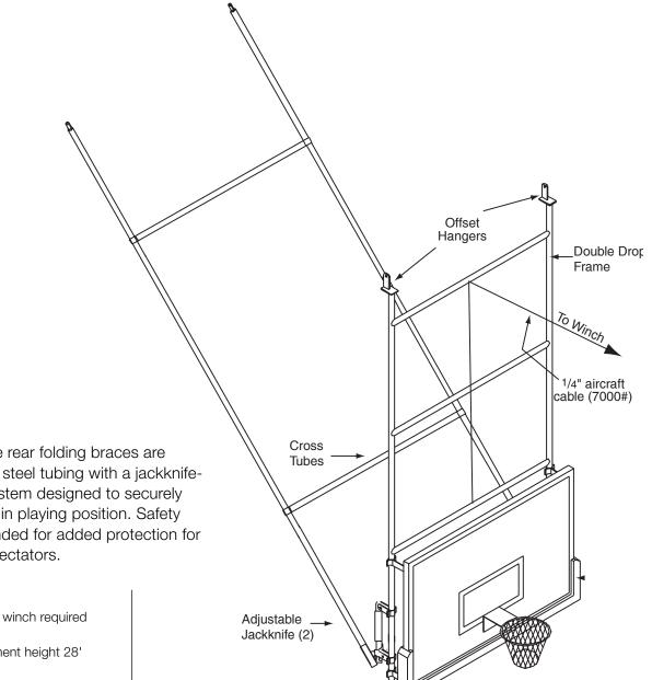
Fully adjustable rear folding braces are constructed of steel tubing with a jackknifetype folding system designed to securely hold backstop in playing position. Safety belt recommended for added protection for players and spectators.
